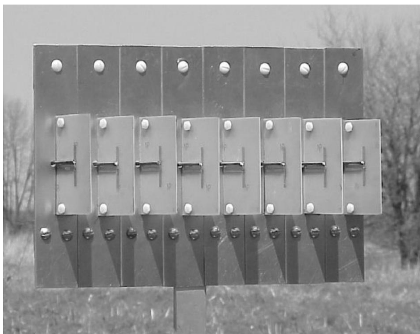
Fig. 1. Photograph of an eight-element linear array of printed dipoles.
