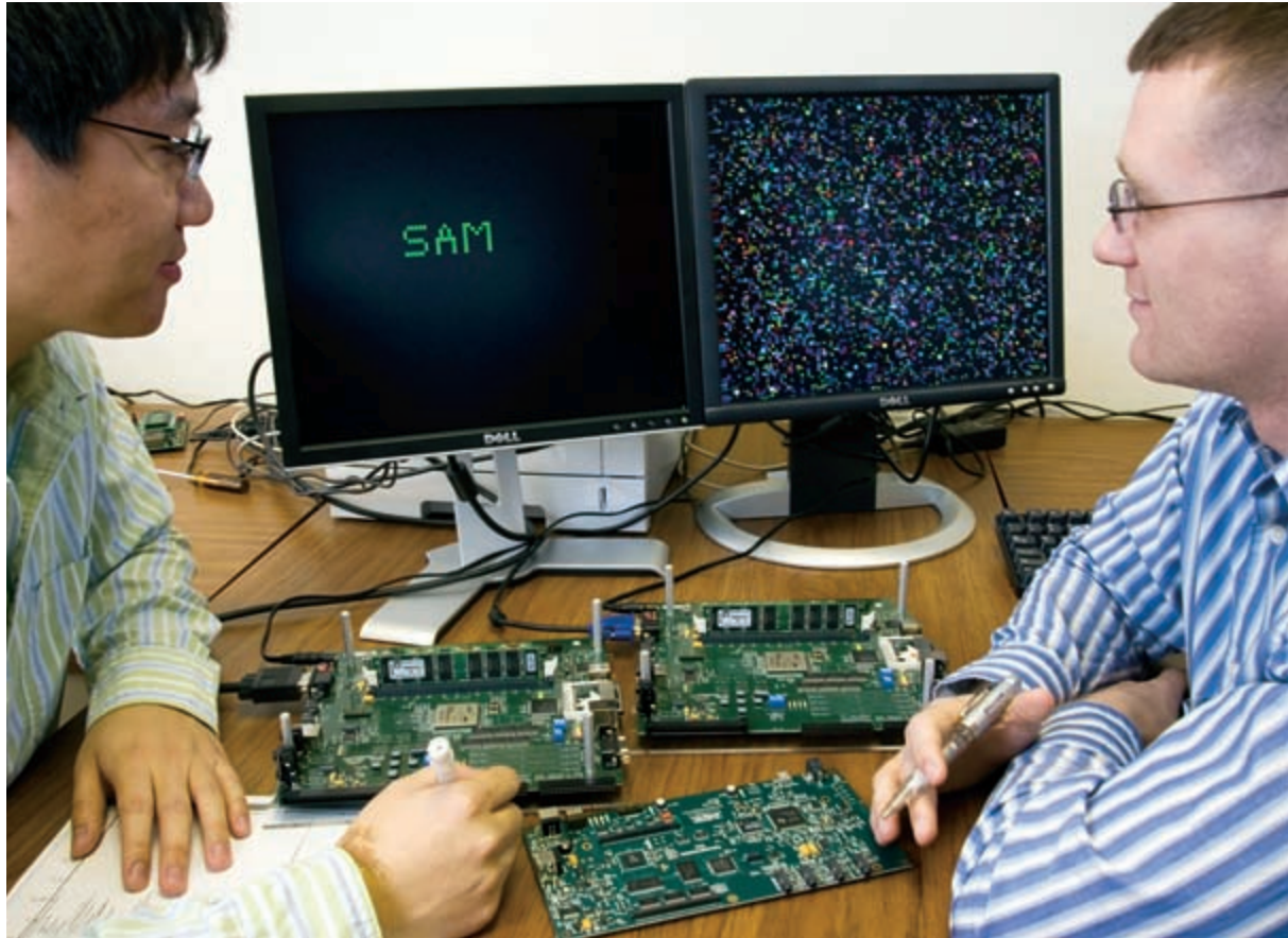
Pengyan Yu (left) and Eric Simpson demonstrate SAM (secure authenticated mode). Unauthorized devices see only the noise on the right, while the authorized device sees the magic word.
