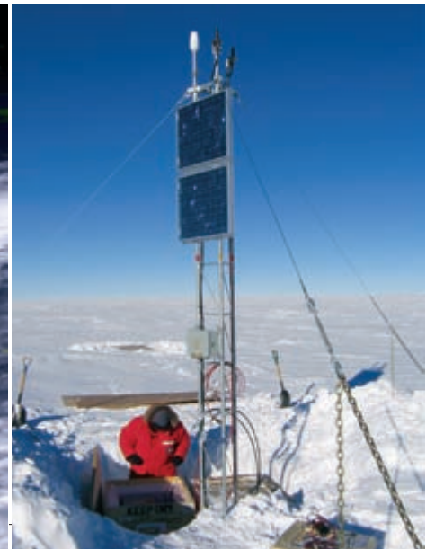
Scott Bailey is deputy principal investigator of NASA's AIM mission. Right: At South Pole Station—testing a prototype of an instrument that will help map the electrical current systems that are driven by solar wind and the magnetosphere.
