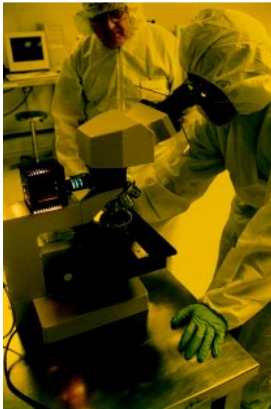
Facing page: Robert Hendricks, director of Virginia Tech's microelectronics task force, monitors air quality in the new microchip fabrication clean room. The laboratory was built as a Class 10,000 facility, but is maintained as a more stringent Class 1,000 operation. Left: A student in the new laboratory checks a device structure under an optical microscope.
