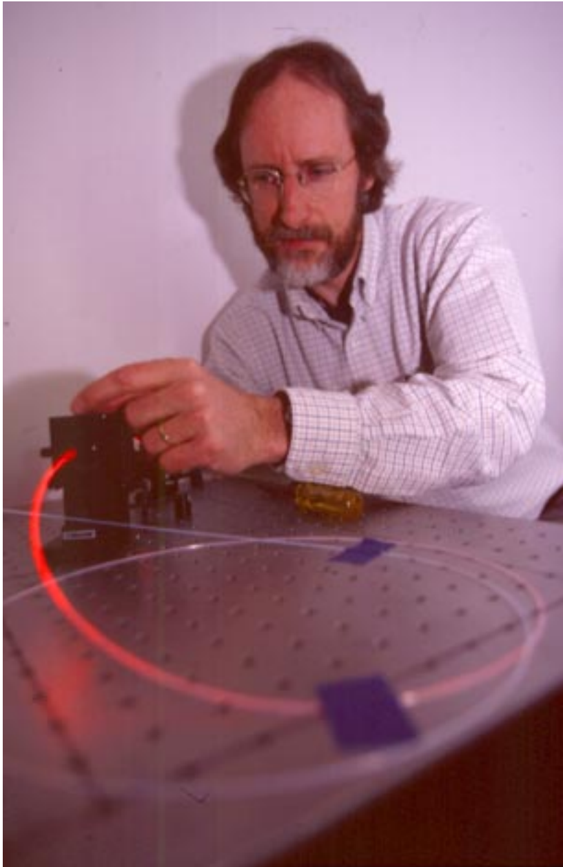
Left: Russell May, president of Prime Photonics, aligns a sapphire optical fiber as he prepares to measure the optical losses in the fiber before using it to construct a high-temperature sensor. Right: Anbo Wang, co-founder of Prime Photonics and director of the department's Photonics Laboratory where the sensor technology was developed.
